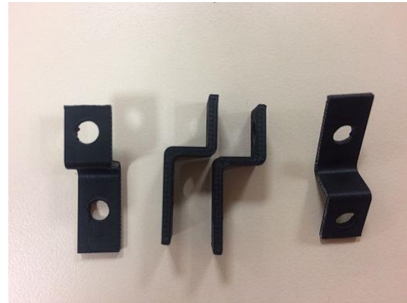
Figure 10b: Pièces 3D imprimées
