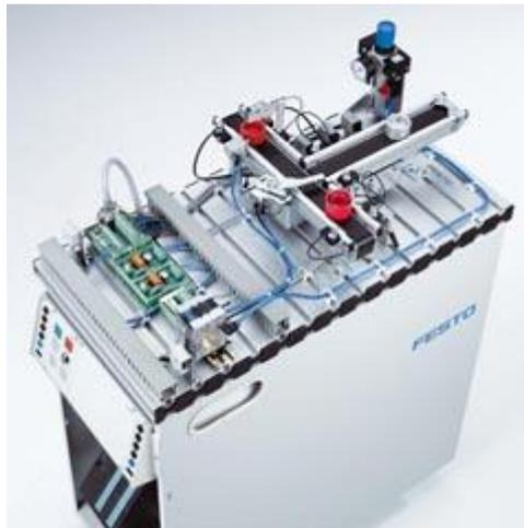
Figure 1: Modular Production System de Festo
